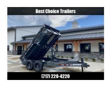
2024 Lamar 7x12' Dump Trailer 14000# GVW \* DROP AXLES \* HD AXLE BEAM \* REAR JACKSTANDS \* 17.5 16-PLY TIRES \* OIL BATH HUBS \* 12" O.C. C/M \* 7GA FLOOR \* TARP KIT \* SCISSOR HOIST \* 12K JACK \* CHARCOAL \* RIGID RAILS \* HD COUPLER \* NESTLED I-BEAM FRAME
