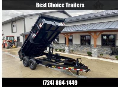
**2024 Big Tex Trailers 14LP 7x14' HD Low Profile Dump Trailer 14000# GVW \* DEXTER AXLES \* SCISSOR HOIST \* 8" I-BEAM FRAME \* UNDERMOUNT RAMPS \* COMBO GATE \* 12K JACK \* 24" 10 GA SIDES \* TARP KIT \* REAR STABILIZER JACKS**
