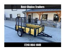
2024 Sure-Trac 5x8' High Side Utility Landscape Trailer 2990# GVW \* 24" 3-BOARD HIGH SIDE \* 2" TUBE TOP RAIL \* 2X2" TUBE GATE C/M + SPRING ASSIST + FOLD FLAT \* TOOLESS GATE REMOVAL \* SPARE MOUNT \* PROTECTED WIRING \* SET BACK JACK \* TRIPLE TUBE TONGUE \* D-
