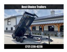
2021 Lamar 7x14' Dump Trailer 16000# GVW \* DEXTER 8K AXLE UPGRADE \* OVERSIZE 6X21.5 11-TON SCISSOR HOIST \* DUAL 12K JACKS \* 7GA FLOOR \* 17.5" 16-PLY TIRES \* SPARE TIRE \* JACKSTANDS \* TARP KIT \* CHARCOAL \* RIGID RAILS \* NESTLED I-BEAM FRAME 28" H \* 12" O.C
